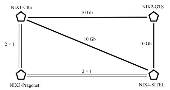
The backbone platform is a series of CISCO 6500 switches. In the NIX1, NIX2 and NIX4 nodes, connection lines with a throughput capacity of up to 10 Gb/s are supported. NIX3, whose utilisation is the lowest, is an exception; its switch only enables connection lines of up to 1 Gb/s.
